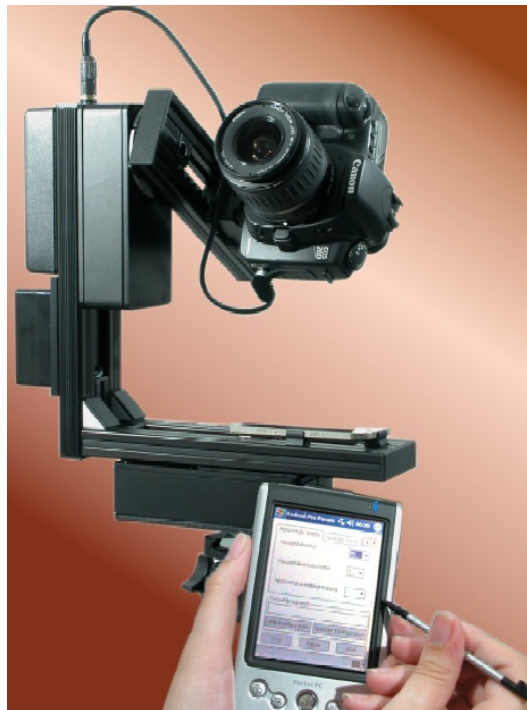
Figure 7.4: Automated panorama head. (Source: Wikipedia https://commons.wikimedia.org/wiki/File:Rodeon_vr_head_01.jpg )
